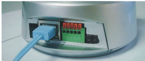
Figure7 Connecting the Ethernet wire
